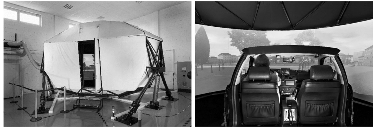
Fig. 1 Setup of the driving simulator with the motion platform and the dome (left) and the mock-up inside the dome (right)
